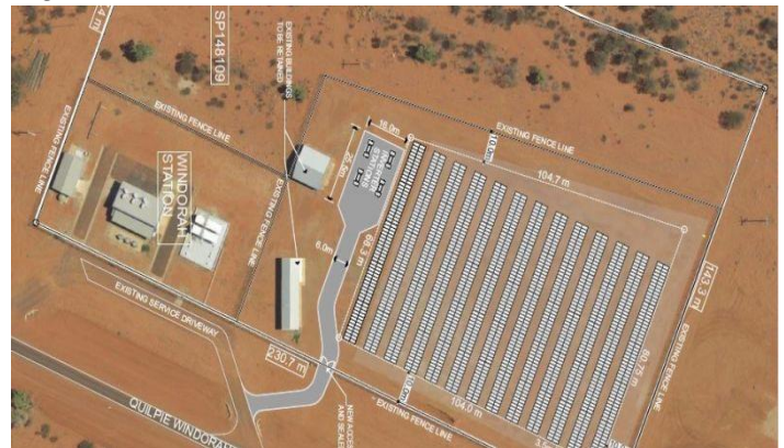
Fig 5 – The proposed layout of the new solar farm and battery facility adjacent to Windorah’s existing power station.
